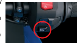
Cruise control system switch
